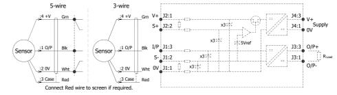
Putting Into Service: The sensor must be used with a galvanic isolation barrier designed to supply the sensor with a nominal 5V and to transmit the sensor output to a safe area. The barrier parameters must not exceed:
